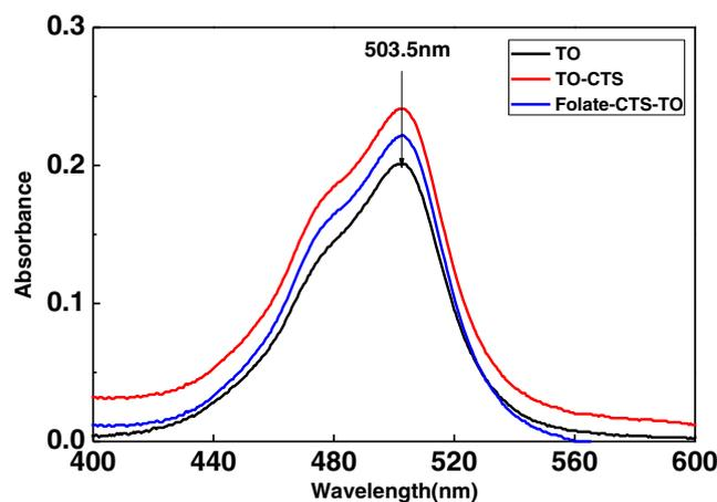
Fig. 3 UV spectra of TO and its derivatives, spectra of aqueous solution with the concentration of 2 mg·L<sup>-1</sup>
