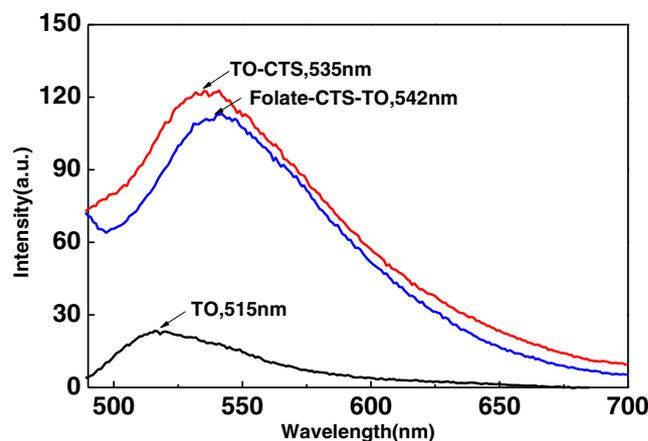
Fig. 4 Fluorescence spectra of TO and its derivatives, spectra of aqueous solution with the concentration of 3 mg·L<sup>-1</sup>
