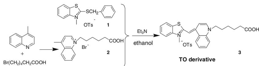
**Scheme 2** Synthetic routes of fluorescence probe FA-CTS-TO complex
